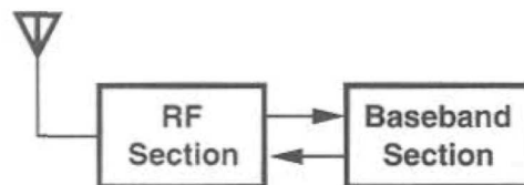
Figure 1.3 RF and baseband processing in a transceiver.
