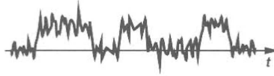
Figure 2.20 Binary signal corrupted by noise.
